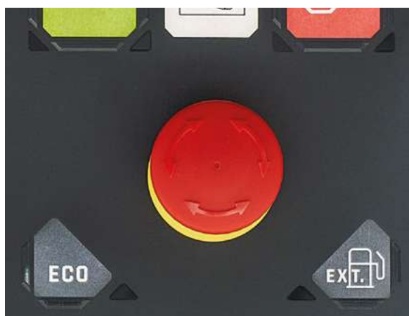
Activation of ECO mode and external refueling
