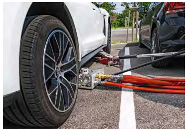
If necessary, the vehicle can be raised with a jack or hydraulic spreader.
