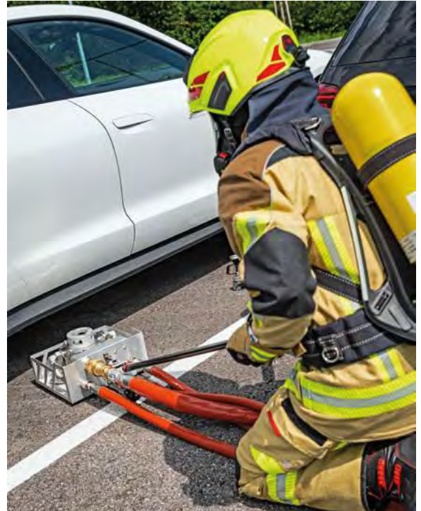
The extinguishing unit is positioned on the battery.
