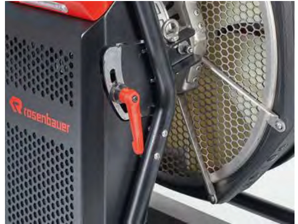
Nozzle adjustment lever from -10^{\circ} to +20^{\circ}
